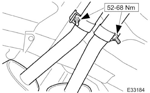
3. Correctly position the intermediate mufflers to the front muffler to align the correct reference / index indicator ring.
