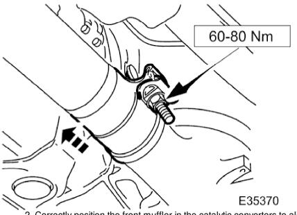
2. Correctly position the front muffler in the catalytic converters to align the correct reference / index indicator ring..
