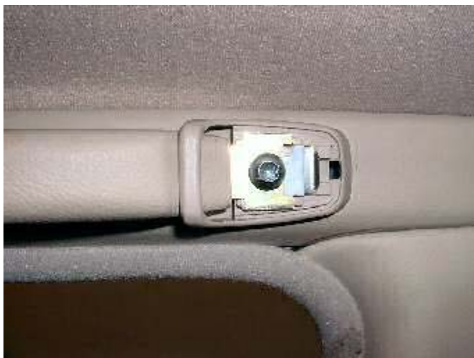
To remove the pull handles, pry the metal trim up and out at the end of the handle. It pops right out.
