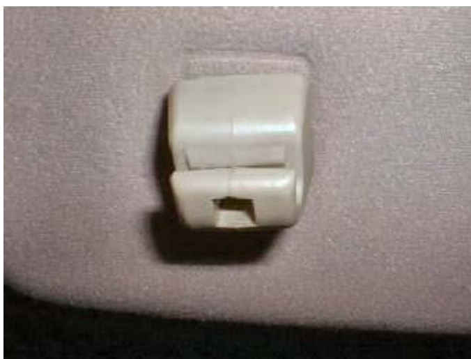
Remove the visor screws and this support on the opposite end of the visor. It has a phillips head screw holding it on (can be removed through the hole).
