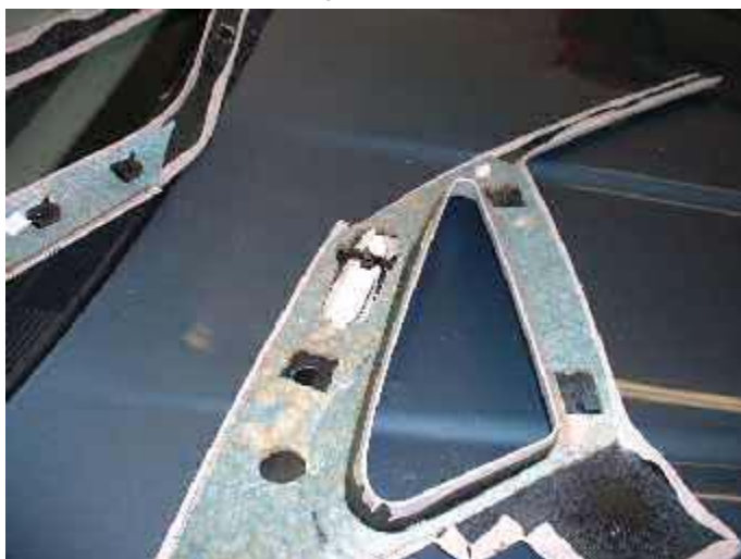
The side trim is attached with small plastic plugs. You can see the black plastic plugs in this picture. To remove them, give them a tug and they should come loose once you've removed the pull handles. It is only necessary to remove one of the rear panels, the other side of the headliner board can be slid from under the panel.
