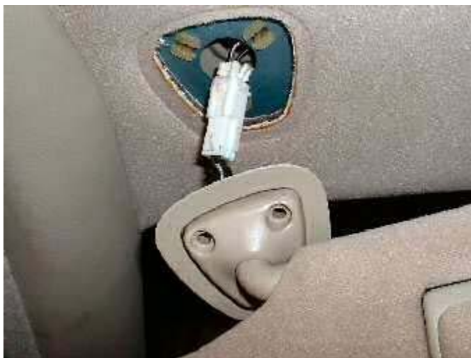
This shot shows the Jaguar XJ8 visor electrical plug
