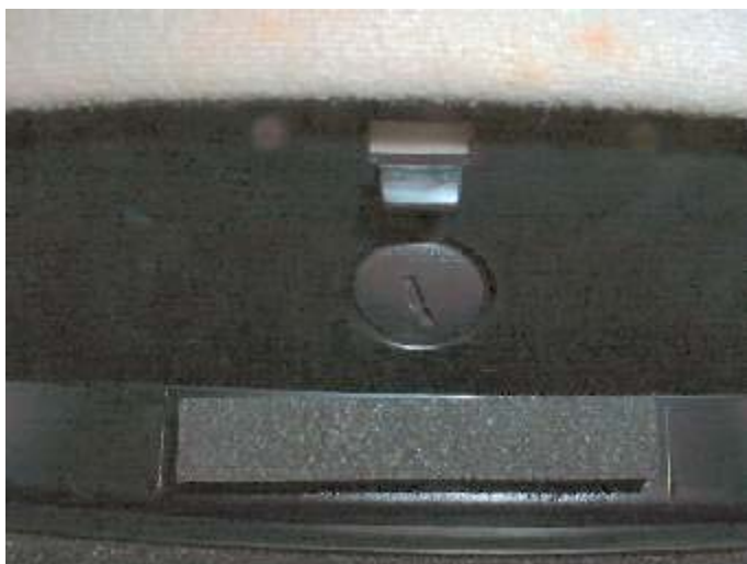
To remove the console, flip the sun visor holder down and use a screwdriver to twist the plug you see in this pic.
