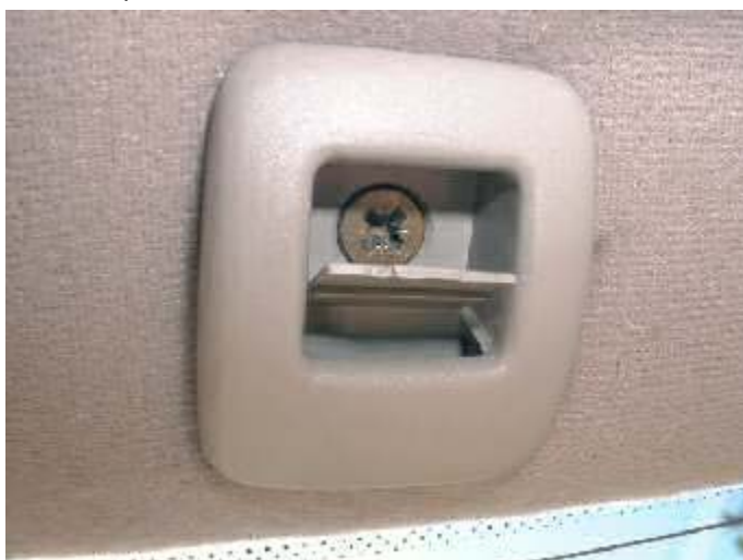
This is a shot of the plastic pieces at the rear of the headliner board, don't know exactly what they are for, but they must be removed. A phillips head screw can be seen once the small plastic cover is pulled up.
