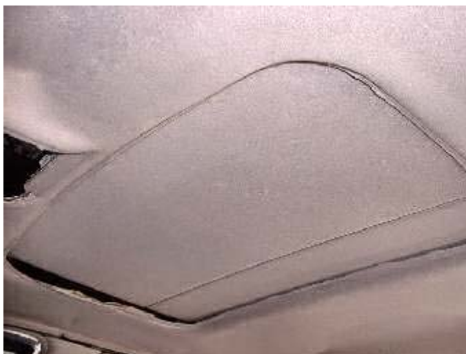
Remove the pinch welt from around the sunroof opening.
