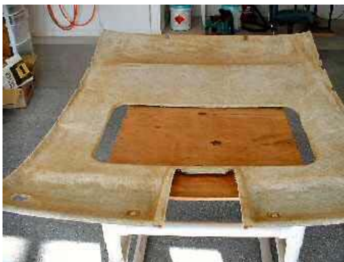
The headliner board of the 1998 Jaguar XJ8 after it has been cleaned. It's ready to be recovered.
