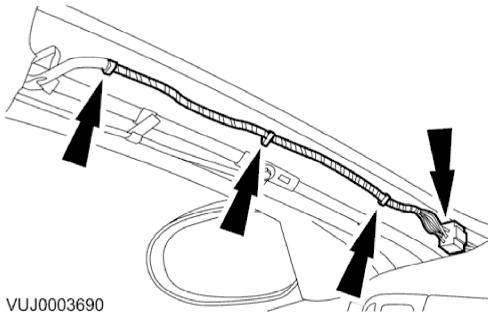
4. Disconnect the left-hand electrical connector and detach the wiring harness.
