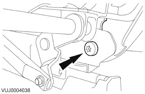
5. Detach the safety belt lower anchor from the underside of the seat.
