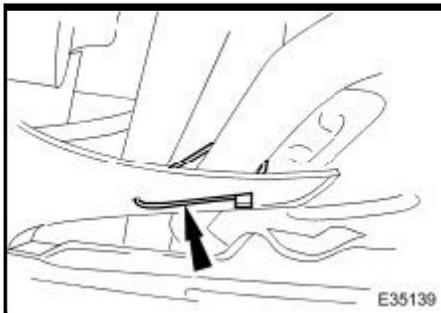
4. At each side of vehicle, remove and discard scrivet securing undertray to wheelarch liner.
