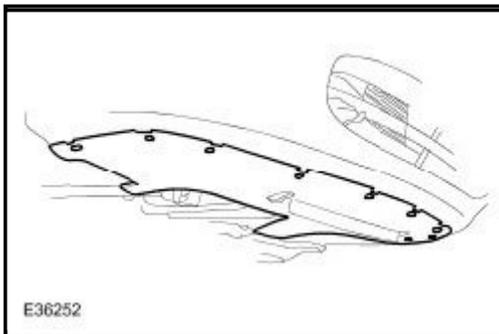
3. Remove and discard tiestrap securing undertray to crossbeam front brace.
