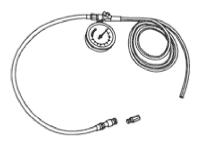
E36466 Test Equipment - Fuel Pressure Relief 310-058 (TE 7635A or JD 209)
