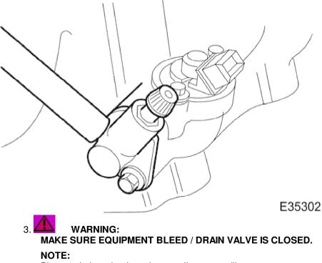
Place a cloth under the valve to collect any spillage.
