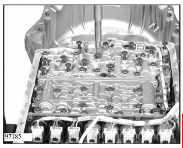
Put the detent disc in the neutral position. Align the control unit, move it into position by hand, and fasten it with 17 machine screws 27.400, and 5 machine screws 27.410.
