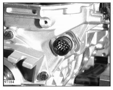
Press in the socket outlet and secure with retaining clip.
