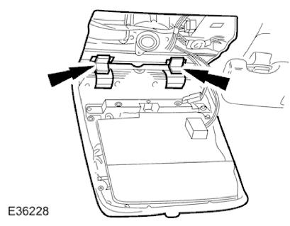
5. Release roof console from retaining clips and remove from vehicle.
