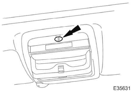
3. Rotate fastener 1/4 turn to release console.
