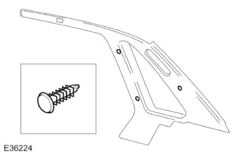
6. Remove the C-pillar trim panel and discard the fir tree fasteners.
