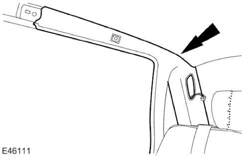
5. Detach the C-pillar trim panel fir tree fasteners from the BIW.
