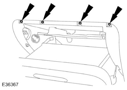
2. Supporting the glovebox, slacken and remove the four top securing screws.
