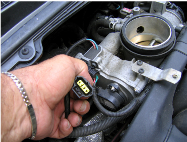
Found that the plug stays were broken
