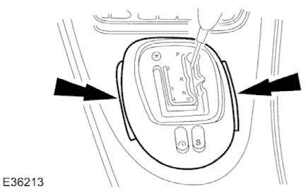
2. Using a screwdriver in the slot in front of the finisher, carefully lift the finisher and ease it from the 'J' gate surround.
