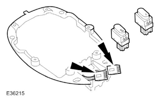
6. Position retaining panel for access, disconnect SPORT mode and cruise control ON/OFF switch multiplugs and remove retaining panel complete with switches.
