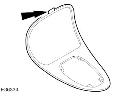
8. Carefully withdraw veneer panel, releasing front locating tongue from upper slot in comsole.
