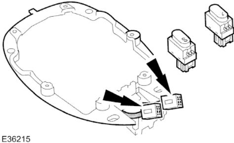
3. Position retaining panel for access, disconnect SPORT mode and cruise control ON/OFF switch multiplugs and remove retaining panel complete with switches.
