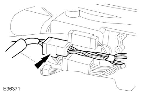
7. Disconnect air conditioning panel flying lead multiplug (blue) in LH side of transmission tunnel.
