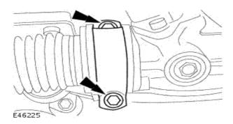
3. Remove the left-hand steering gear mounting bracket retaining bolts.
