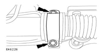
2. Loosen, but do not remove, the right-hand steering gear mounting bracket retaining bolts.
