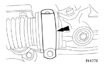
4. Remove the left-hand steering gear mounting bracket.
