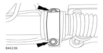
8. Remove the right-hand steering gear mounting bracket retaining bolts.
