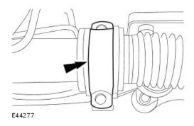
9. Remove the right-hand steering gear mounting bracket.
