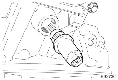
A coolant drain plug is located at the rear of the cylinder block.
