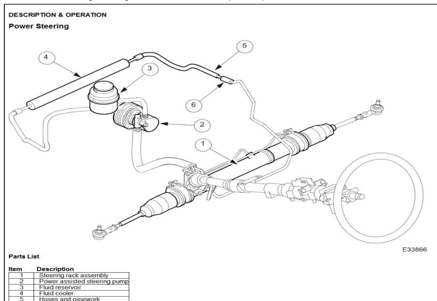
The power steering system is a rack and pinion design, with an engine-driven pump providing the steering assistance.
