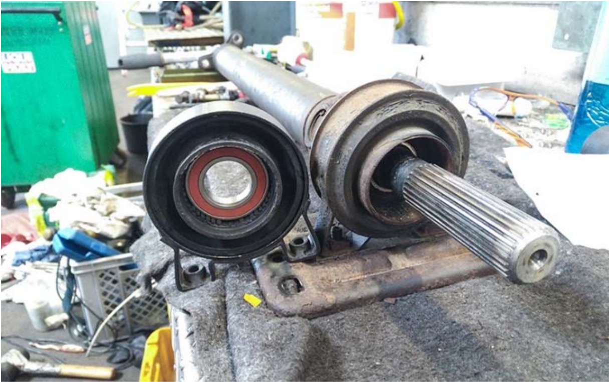
Location: none, old vs. new center support bearing
