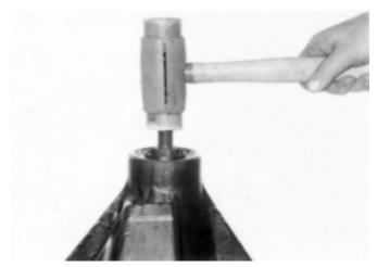
**Figure 3-13**Step (18) Remove pinion by tapping with a rawhide or plastic hammer. Catch the pinion with your hand to prevent it from falling and being damaged.
