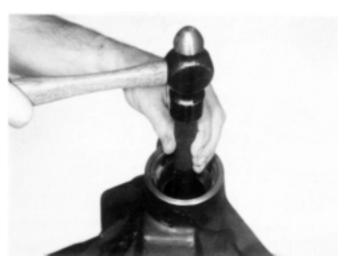
**Figure 3-16**Step (21) Remove the inner bearing cup with tools as shown.
