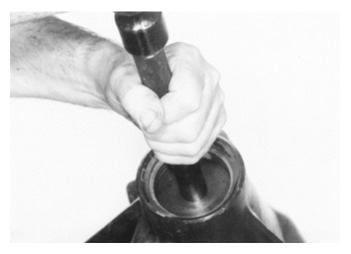
Figure 3-22 Step (24) Assemble the outer pinion bearing cup into carrier as shown. Make sure cup is seated.
