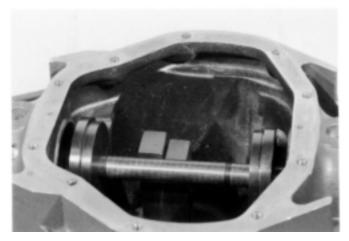
**Figure 3-26**Step (28) Place pinion height block on top of the button end of the pinion gear and against arbor as shown.
