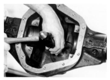
Figure 3-30 Step (32) Place the required amount of shims (and baffle if used) in the inner bearing bore. Drive the inner bearing cup into the carrier. Make sure cup is seated.
