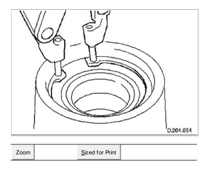
1. Fit outboard circlip to the vertical link.
