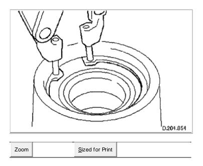
9. Using special pliers remove and discard outboard circlip from the vertical link.
