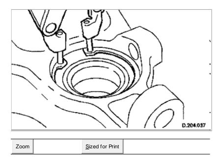
8. Using special pliers remove and discard the inboard circlip from the vertical link.
