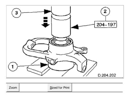
10. Using a hydraulic press, remove wheel bearing from vertical link.
