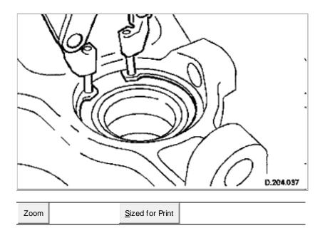
4. Fit inboard circlip to the vertical link.
