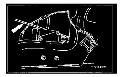
8. Disconnect lock motor link rod.
