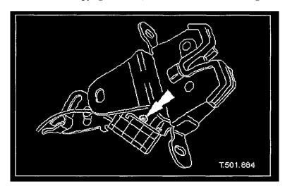
9. Withdraw lock assembly from trunk, release trunk open switch retaining tang and remove switch from lock assembly.
