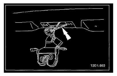
7. Disconnect lock barrel link rod.
