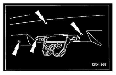
4. Release and discard the four trunk lid liner rear fasteners and position liner for access.
