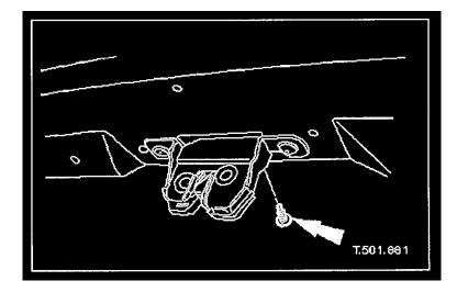
6. Remove the latch assembly securing bolt.
