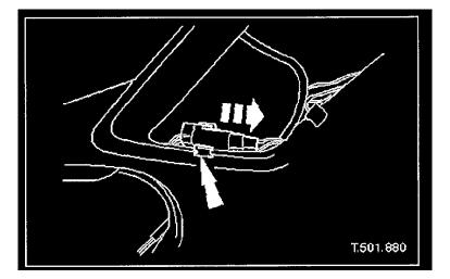
5. Release trunk open switch multiplug from retaining clip and disconnect multiplug.
