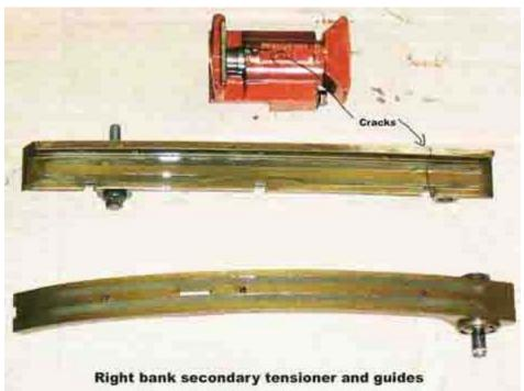
Though the tensioners of this 1998 XJ8 engine with 56,000 miles appeared intact on visual inspection with the valve covers removed, upon disassembly both were discovered to be badly cracked, and so was one of the main tensioner guides. A cracked tensioner can break apart and cause cam chain failure, damaging the engine severely.
