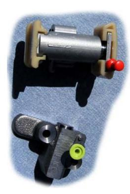
Jaguar's third-generation secondary and primary tensioners are mostly metal, not plastic. Although we have not had problems with the second-generation plastic units, as of April 2005 we are using third-generation tensioners exclusively.
