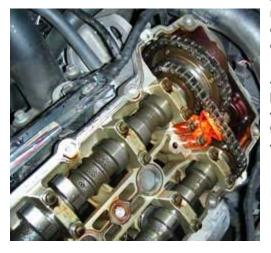
The secondary tensioner (red) for each cylinder bank is visible when the valve cover is removed.
