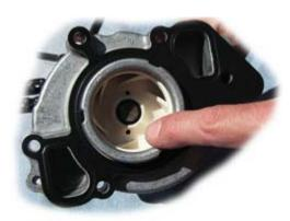
Jaguar's original water pump design was faulty, resulting in broken ceramic impeller blades and engine overheating. The improved unit (above) is far more reliable and highly recommended if your car still has the original.
