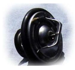
Thermostats should be replaced at least every two years on late-90s Jaguar V8 cars. Worn units can cause secondary problems that are not immediately traceable to the thermostat unless the technician has experience spotting the tell-tale indicators.
