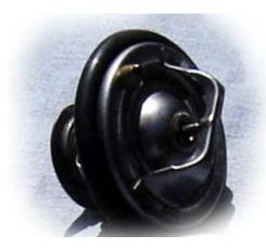
Thermostats should be replaced at least every two years on late-90s Jaguar V8 cars. Worn units can cause secondary problems that are not immediately traceable to the thermostat unless the technician has experience spotting the tell-tale indicators.
