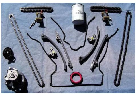
Depending on your needs, we can replace only the secondary tensioners, or as shown above, the primaries, secondaries, chains and guides. At the bottom left are replacement water pump and thermostat, another weak point on early Jaguar V8s.
