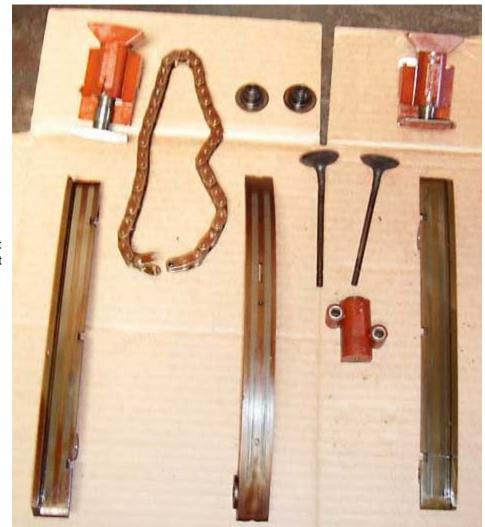
When the worst happens: This 1999 XJ8's tensioners both cracked. When the one at the top left broke, its timing chain (shown) snapped and the valves collided with the pistons. Two of the bent valves are shown in this photo. Though such damage requires significant shop time to repair, engine replacement is usually NOT indicated, and the parts required are reasonable in quantity and cost.
