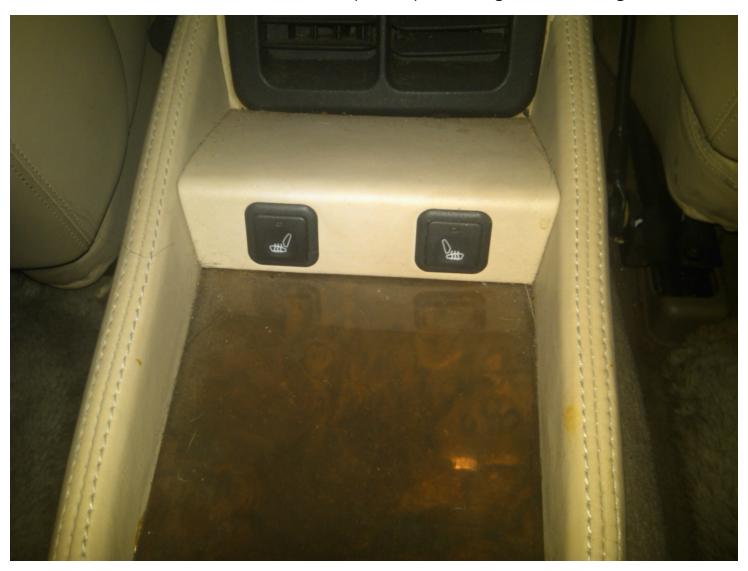
STEP-2 Pry the FRONT edge of the shelf plate and pull forward-out
