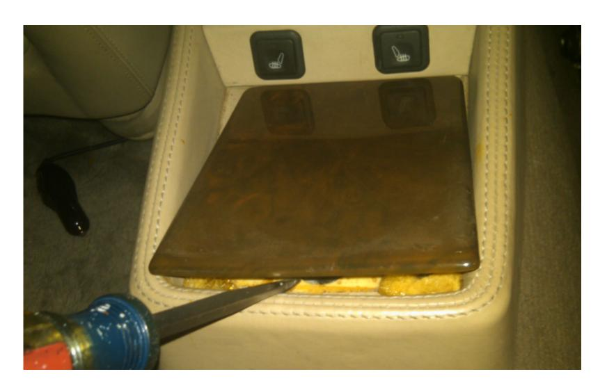
STEP-3 Remove the 2 phillips screws and remove the console
