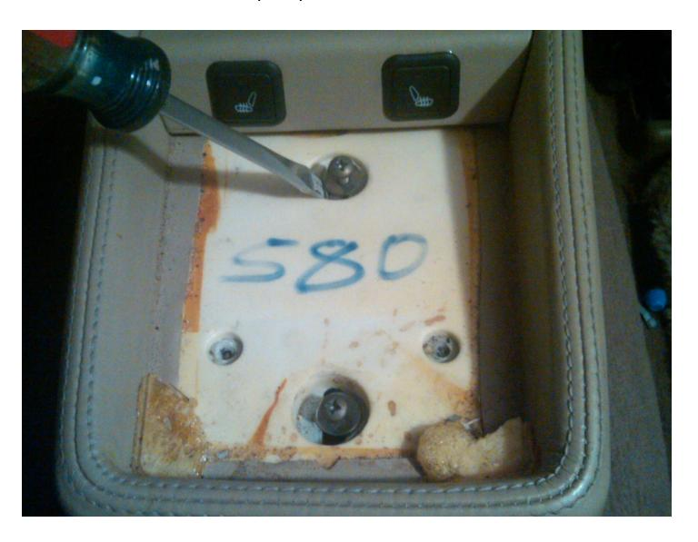
STEP-4 Push the retaining clip in an push the entire unit out the front
