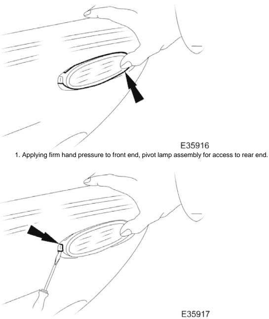
2. Exercising care to avoid damaging paintwork, use a small screwdriver at rear end of lamp, to press and release retaining tang.
