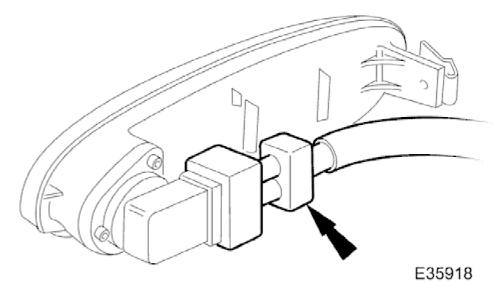
3. Withdraw lamp from bumper for access and disconnect harness multiplug.
