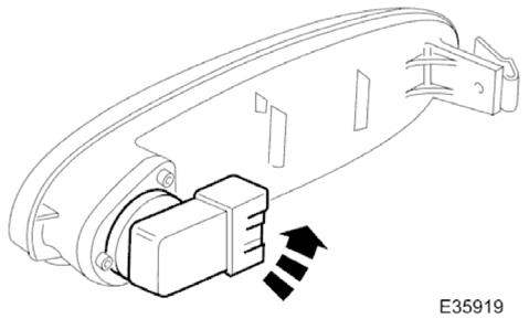
4. Rotate bulb holder 1/4 turn counter-clockwise to release it from lamp assembly.
