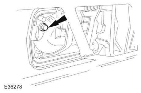
11. Holding handle firmly in position, slacken and remove front securing bolt and remove handle assembly from door.
