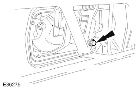
8. Slacken and remove outer handle rear securing bolt.
