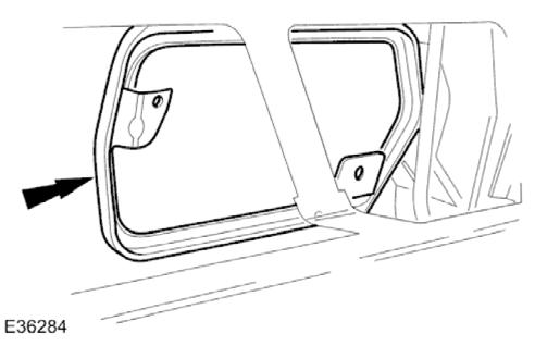
12. Remove door handle clamping plate.
