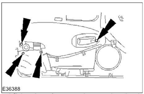
3. Slacken and remove four screws securing armrest to door casing and remove armrest from casing.
