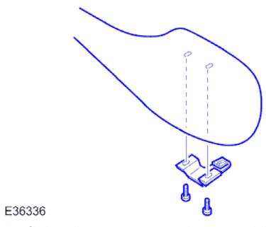
5. Slacken and remove two screws securing armrest retaining clip and remove clip from armrest.
