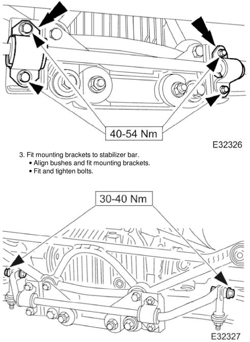
4. Tighten nuts securing stabilizer bar to links.
