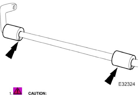
Make sure the Castrol NTR grease is only applied to the inner surface of the mounting bushes. Failure to follow this instruction may affect the retention of the bushes in the retaining brackets.
