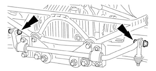
2. Remove nuts and bolts securing stabilizer bar to links.
