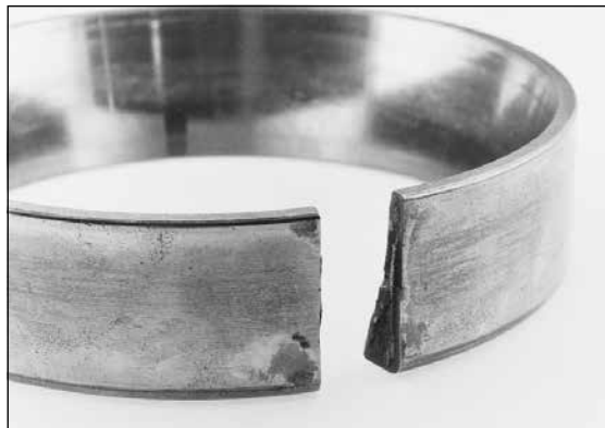
Fig. 51. This is what happens to a cup that is loose in a wheel hub. The cup turns and wears the cup seat so the fit becomes more loose. Then the cup starts to stretch or roll out. The cup, as it rolls out, continues to wear the cup seat and the cup continues to stretch. This process continues to the point where the stretch of the metal reaches the breaking point and the cup cracks open.
