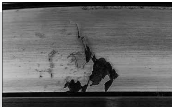
Fig. 23. Misalignment, deflections or heavy loading on this tapered roller bearing caused GSC spalling.
