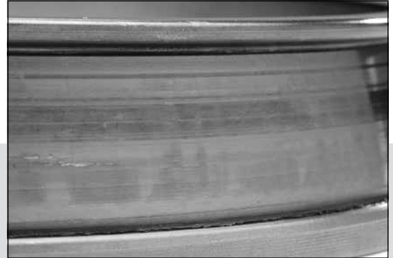
Fig. 17. Level 1 – Discoloration due to elevated operating temperatures.
