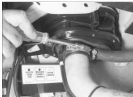
7.6 Remove the clamp that retains the fuel filler assembly to the filler neck
