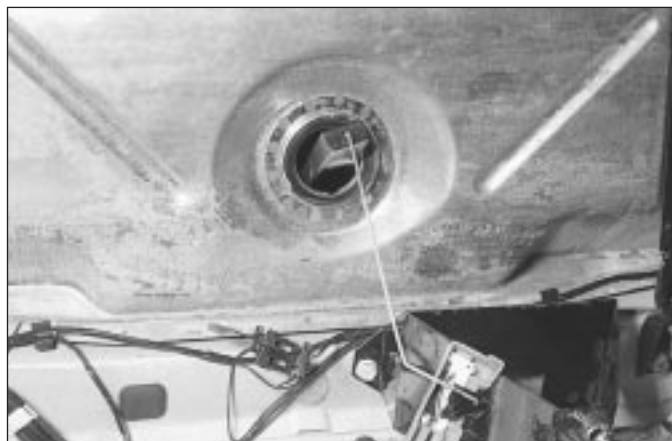
5.11 Lift the fuel level sender unit assembly from the fuel tank at an angle so as not to damage the float or arm
