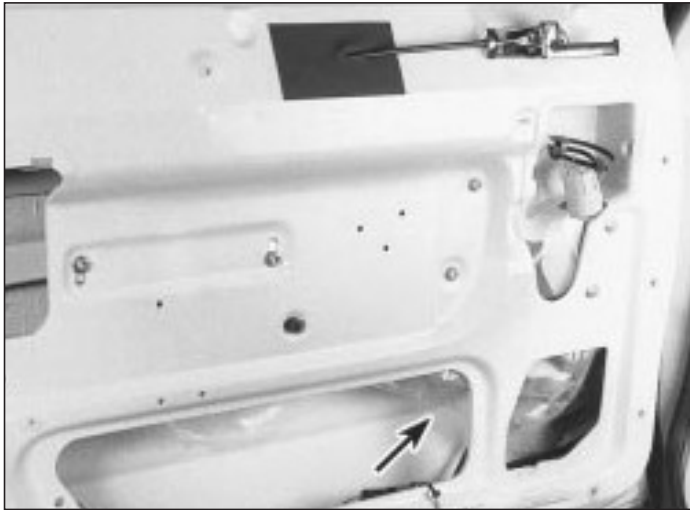
19.7a Work through the door access hole (arrowed) to remove the hinge-to-door retaining nuts from inside the door
