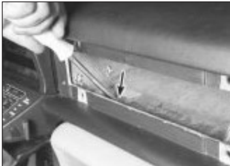
24.8 Remove the retaining screws in the air conditioning duct opening
