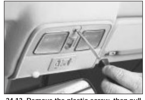
24.13 Remove the plastic screw, then pull the overhead console down and unplug the electrical connectors
