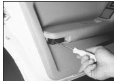
18.7b Remove the retaining screw from inside the lamp housing
