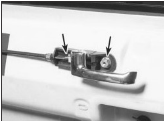
20.13 After removing the cable from the latch assembly, detach the handle retaining bolts, then pull the handle and cable assembly free from the vehicle
