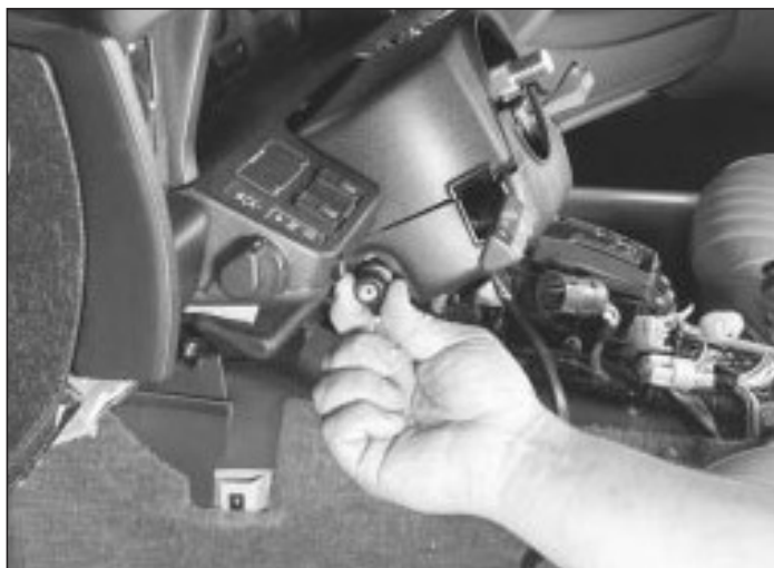
27.2 Pull off the knob from the instrument panel rheostat
