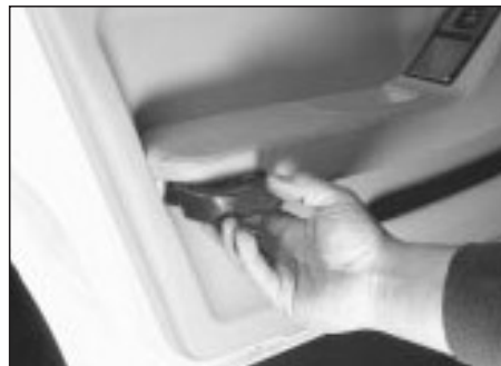
18.7a Prise out the courtesy lamp lens
