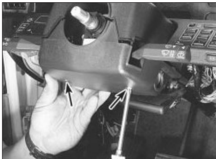
27.3 Remove the lower steering column cover screws
