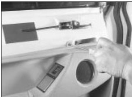
18.6 Detach the screws along the top edge of the lower trim panel
