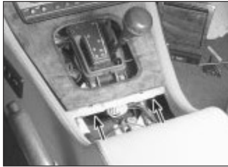
24.4 Working through the ash tray opening, remove the radio trim bezel wingnuts (arrowed) located under the trim bezel
