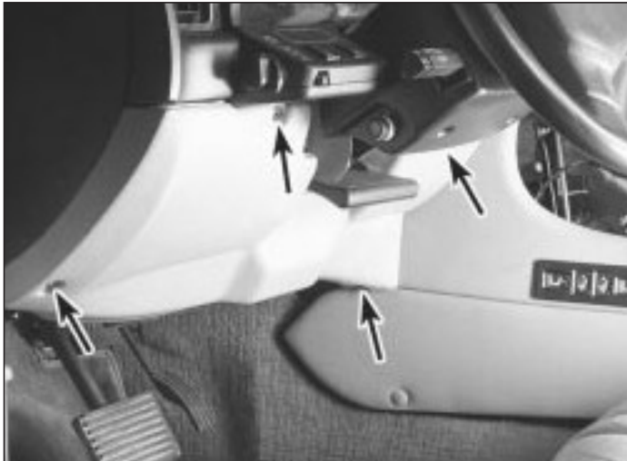
26.2 Remove the retaining screws along the outer edge of the knee bolster, then remove it from the vehicle
