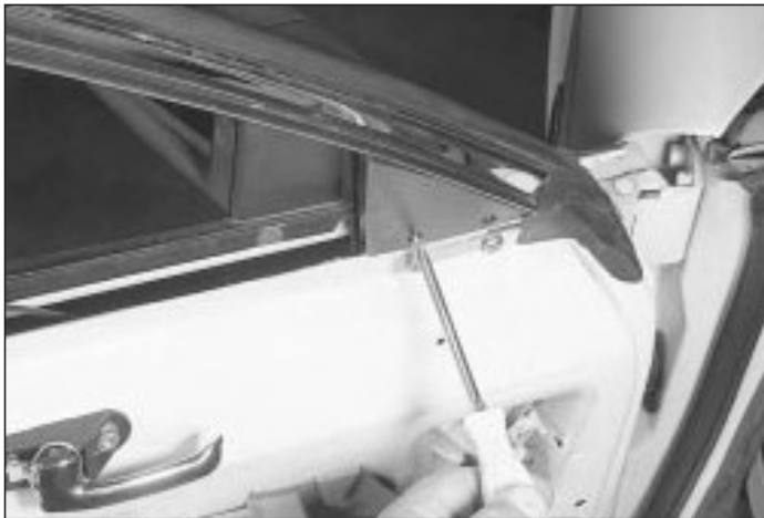
23.2 Remove the trim cover retaining screws
