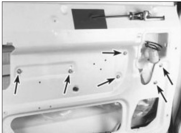
21.3 Detach the window regulator bolts (arrowed)
