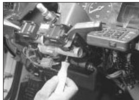
27.4 Remove the four screws securing the upper half of the steering column cover
