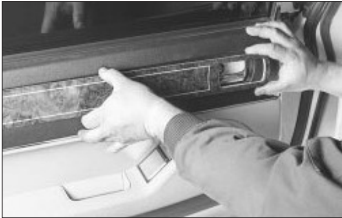
18.4 Gently prise out the clips securing the wood finish panel
