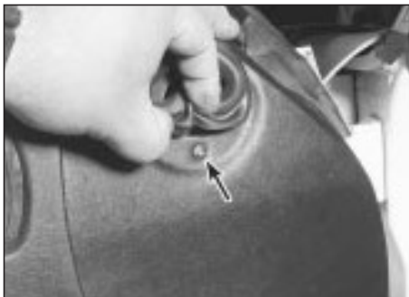
18.2 Lift the air duct-to-body seal to access the trim panel retaining screw (arrowed)
