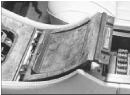
24.3b Pull the ash tray towards the rear of the vehicle to remove it - don't pull it straight up
