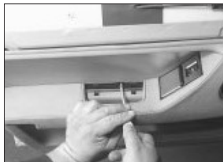
18.8b Remove the screws behind the armrest/pull handle trim cover
