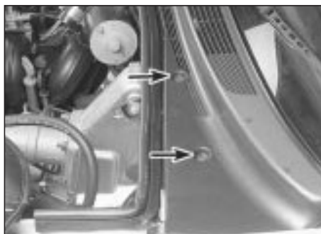
28.2 Remove the screws (arrowed) located along the top of the cowl cover
