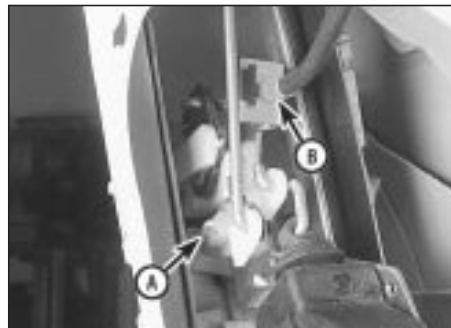
20.2 Detach the outside handle-to-latch rod (A), then remove the inside handle-to-latch cable (B)
