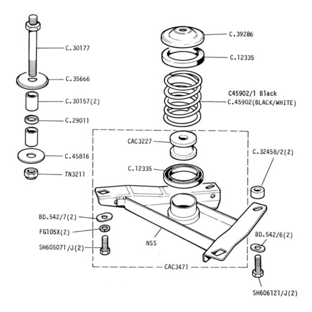
This is the 6cyl Transmission mount Parts Drawing.
