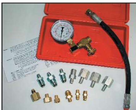
(3) We picked up an inexpensive power steering pressure tester, which is just a high-pressure gauge, a length of hose, and a fitting assortment.
