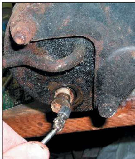
(6) If the valve doesn't drop out in your hand when you remove the fitting, use a magnetic tool and it'll come right out. If the large spring behind it drops out, too, just shove it back in. Note: There's no need to remove the pump from the car.
