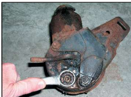
(4) Unscrewing the pressure fitting from our prize (7/8" hex), we discovered...
