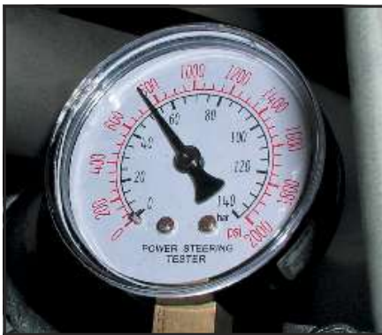
(11) We swapped in the I6 valve assembly, and the gauge reading dropped to 750-825 PSI. Big change! But it still felt power assisted, and a road test proved the worth of the pressure reduction. No negatives whatsoever! A scrawny 9-year-old neighborhood kid was able to still very easily turn the wheel from lock to lock, with the tires on coarse concrete.
