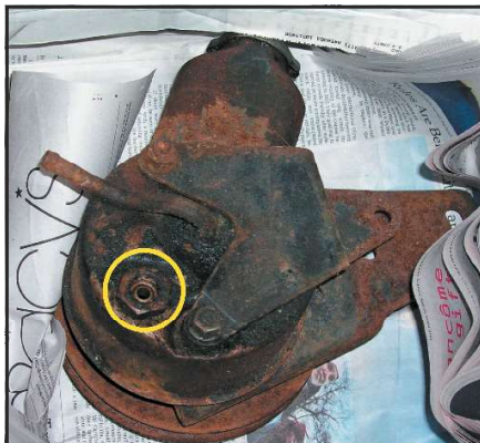
(2) All Saginaw pump have the pressure fitting on the rear (circled), whether built in the '60s or '00s. Metric or USS, round or ham-shaped reservoir all use the same fitting OD threads (which are USS). This is our nasty junkyard slant-six A-body pump, circa late-'60s.
