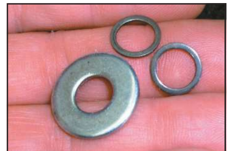
(14) The shims are 3/8" ID, 1/2" OD (exactly, nothing metric here!) A hardware store 3/8" flatwasher (left) has way too large of an OD. You'll need to either grind down the OD (need not be precise), or start with a 1/2" OD washer and drill the center hole to 3/8". If you're shooting in the dark (no pressure gauge), we'd start by adding about 0.062" to whatever you find in your valve. Brass might be easier to work with than steel and would be fine.
