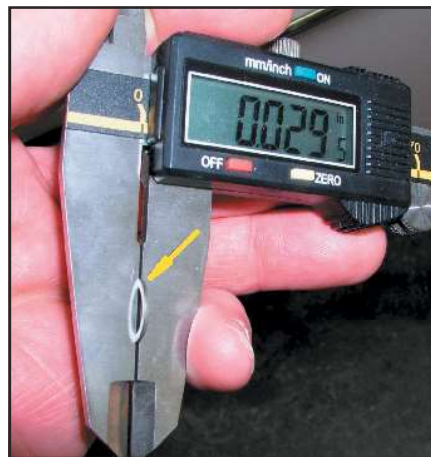
(13) We took the slant-six valve back out, and measured the shim pack. One washer was 0.047", and the second one was 0.030".
