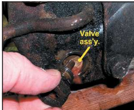
(5) ...some nasty moisture-induced scuzz inside. We hoped the valve would be OK.
