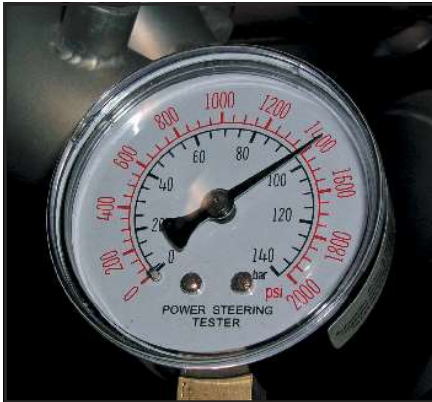
(10) Depending on temperature and RPM, it read between 1375 and 1450 PSI.
