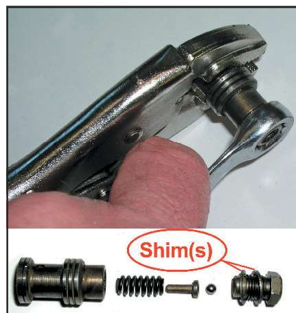
(8) ...we had to have a peek inside. The old FSMs suggest a soft-jaw vise for disassembly, but that's not really practical. We had an old US-made Vise-Grips (got a pair? They are like gold), which fit between the "piston ring" lands (careful, don't damage the machined surfaces). Then the end cap nut comes right off (7/16" hex). Later, we'd discover that all that's needed for a pressure drop is a thicker shim-washer pack...a true zero-buck upgrade!
