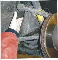
Inspect the spring turrets for rusting. Ensure that the coil springs are not broken or corroded. Check that the shock absorbers are leak-free and free from bounciness. Check all bushes and the top and bottom swivel joints for excessive play.
