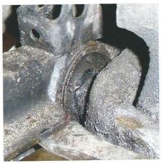
Ensure that the rear radius arms are not severely corroded and that their integral rubber bushes have not disintegrated. Assess the springs, shock absorbers and mountings. Check for wear in the outer, lower fulcrum bearings (pictured).
