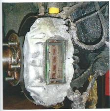
Check all fixed pipework and flexible hoses for corrosion or deterioration. Check the master cylinder and servo for leaks. Check fluid level; replace every two years. Scrutinise the front pads for wear and the discs for wear, corrosion and warping.
