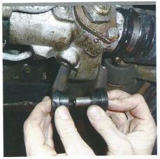
Inspect balljoints for play, gaiters for deterioration and the rack for sloppiness. Pay particular attention to the rack mounting bushes – if they're worn, the rack moves sideways. Check the rack for leaks. Top up power steering fluid with ATF.
