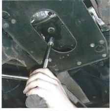
Differential oil Remove the level plug and top up to the base of the aperture. The limited slip differential requires special API GL5 90 LS oil. Renew at least every 20,000 miles. Capacity: 2.75 pints (1.6 litres).
