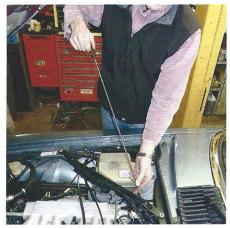
Auto gearbox fluid Check fluid level (consult handbook) and check its colour. If it's brown and smells burnt, the transmission is ailing. Replace with fresh ATF every 20,000 miles. Capacity: 16 pints (9.1 litres).
