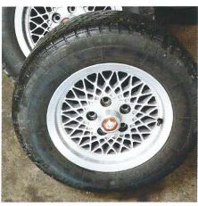
Wheels and tyres Check the aluminium alloy wheels for corrosion and impact damage. The low-profile 15in and 16in diameter tyres don't take kindly to kerbing. Check the tracking if uneven wear is evident.
