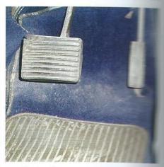
18 Interior aspects Assess pedal rubbers. Test the operation switches, controls and instruments. Instant belts for fraying, and ensure that they later than correctly. Look for rust around mountings.
