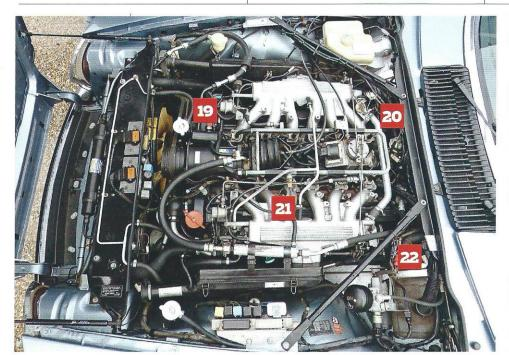
0il leaks Check for engine oil leaks, essential limit the sump plug, the sump itself and the waller cover gaskets.
