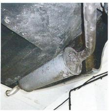
Exhaust system Check the exhaust system for leaks, insecurity, damage and disintegration. Include all the mountings in your examination. The front downpipes are particularly vulnerable to damage.
