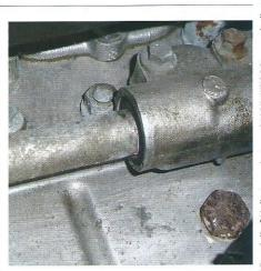
Change coolant every two years or 12,000 miles with red or blue antifreeze. There's a steel pipe passing through a rubber 'O' ring into an aluminium housing on each side of the engine – inspect for leaks. Check the rest of the system for leaks.
