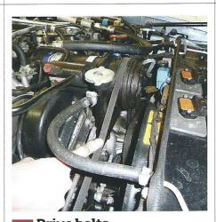
There are four separate belts, serving the alternator, air-conditioning, cooling fan and power steering. Assess condition and tension; renew regardless every 60,000 miles. Remove the power steering belt to access the alternator belt.
