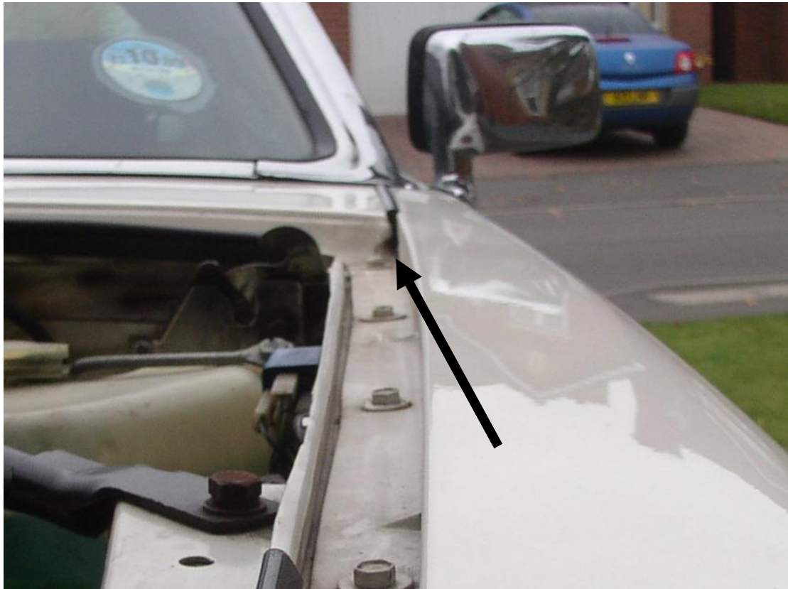
Pic 2 Windscreen pillar drain hole and wing gutter.
