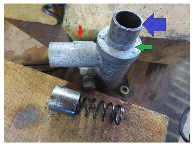
cylinder, the **green arrow** indicates where the cylinder has been released from the outer casing and turned 180 degrees to close the air passage and then resealed; the **red arrow** indicates the air entry tube from the air filter box. The original air passage opening is at the cylinder end of this air passage. The piston has been removed from the unit as is obvious. The following photo shows the air passage at the cylinder end completely sealed with epoxy putty.
