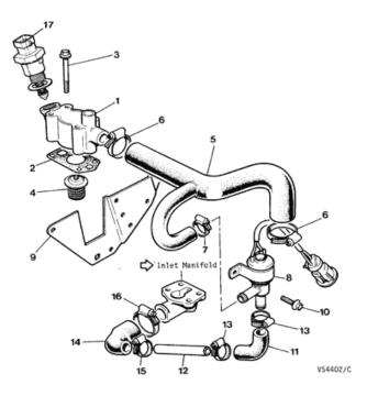
In the diagram, the air inlet is at the side of the solenoid and the outlet to the manifold is at the bottom of the unit. This solenoid flows enough air to enable the V12 to tickover at about 800 RPM when stone sold at an ambient temperature of 0 degrees C (32 F). The photo below shows the unit:
