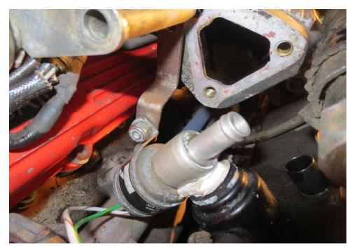
Various pieces of the manifold assembly had to be removed get access to fit the solenoid, but it is quite obvious what to do when you are looking at an actual engine. The following photo shows it all installed and the various bits that had to be removed for access purposes reattached to the B bank manifold. The flexible exit pipe from the solenoid can be seen clearly, linking to the gold steel pipe with a sprung clamp.
