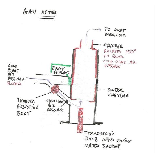
As the diagram shows, the AAV casing has been emptied of its moving parts except for the slow running (tickover) adjustment function. The AAV was then reinstalled on the engine just as before. There is no need to touch the thermostatic bulb.
