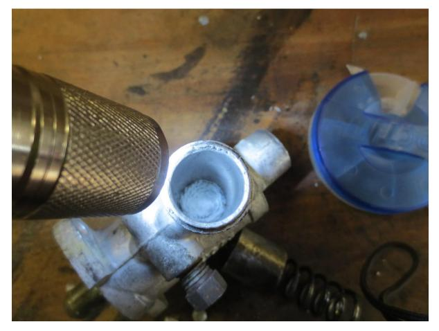
An important point to understand is that blocking this air passage does NOT block the function of the slow running adjustment screw. The air passage for the tickover adjustment has a separate route through the casting. In diagrammatic form, this is what has been done:
