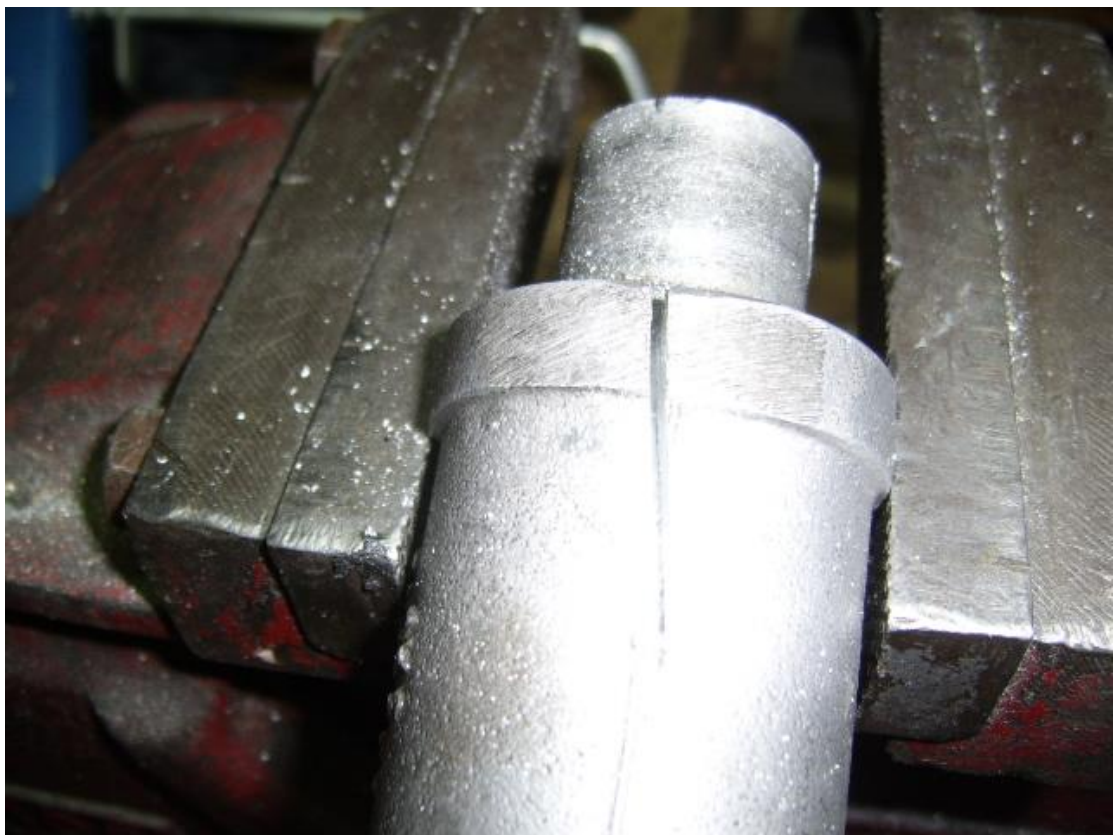
Figure 3 The CUT to release the grip
