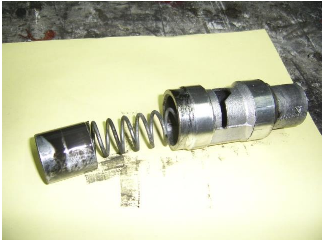
Figure 6 The 3 components of the Tophat
