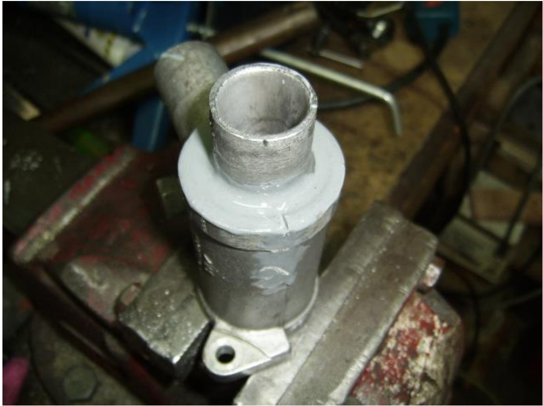
Figure 12 Completed unit with JB weld in place.
