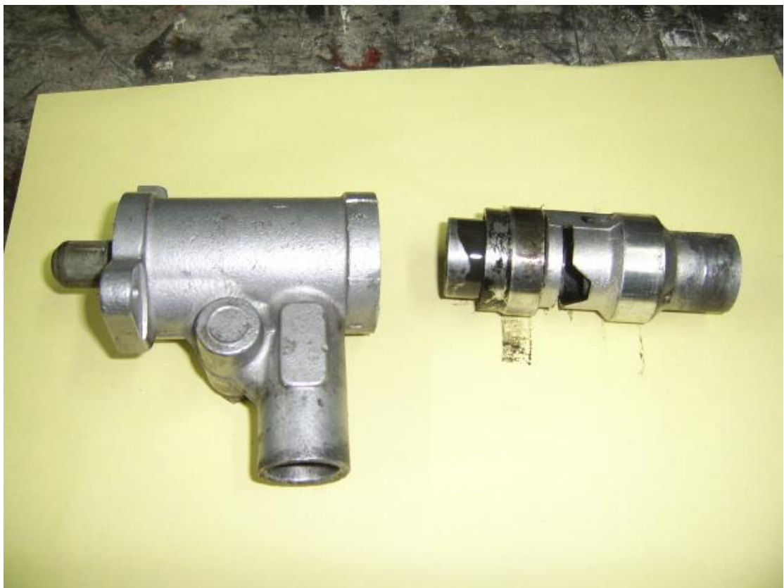
Figure 5 Body on the left and Tophat assembly on the right
