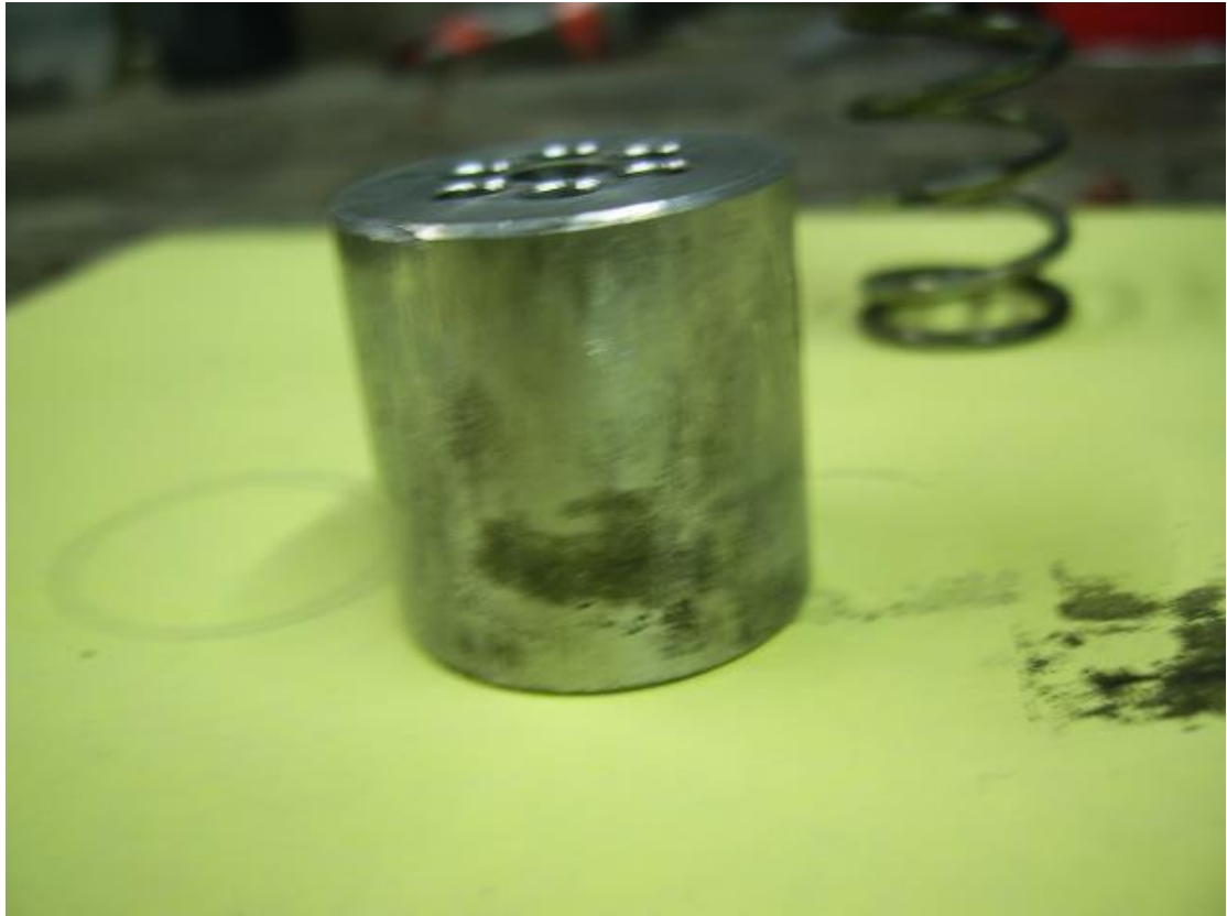
Figure 8 Alloy piston showing scores and carbon build up
