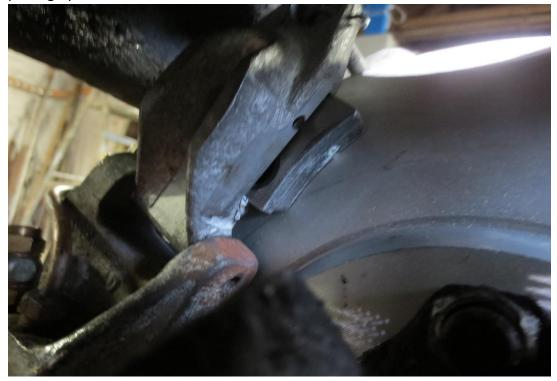
The problem with using this unswept area would be that more than half of the pad would not be directly supported by the calliper, but be "hanging" out of the bottom of it. Whether this would be a problem in practice, as the pad and its backing is bolted to the calliper, is not known. However caution was exercised and a much larger pad was not used in this first stage of modifications. It would be possible to weld an extension onto the calliper arm if testing proves extra pad area is necessary.
