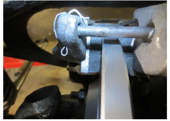
This photograph shows the adjustment screw in position and locked with a split pin:
