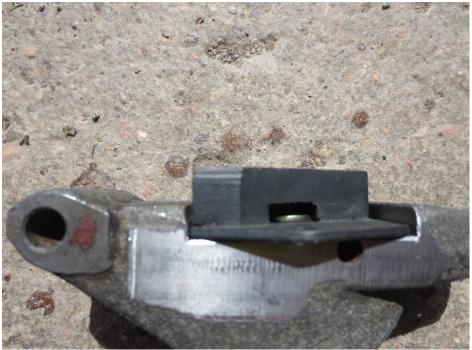
On the replacement pads the backing plate is 6 mm thick, and so quite thick enough to be tapped in order to bolt the pad to the calliper arm. The author replicated the essentials of the original attachment system on the replacement pads, by drilling and tapping the 6mm backing plate of the new pads and bolting them up to the arm with a ¼ inch UNC stainless Allen headed bolt as shown here:
