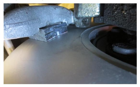
Finally, the automatic adjustment system that compensates for pad wear has a threaded screw that sets the pad position initially. It is then locked into position by means of a split pin that anchors a slot in the screw head to the calliper arm.
