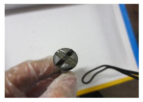
Therefore the screw, which has a coarse thread, has to be adjusted a minimum of half a turn at a time, which is too coarse an adjustment in the author's view, who was aiming for a 5 thou gap at rest between the pad and the disc. The photograph above shows a second slot that was cut in this screw head to allow quarter turn adjustments.
