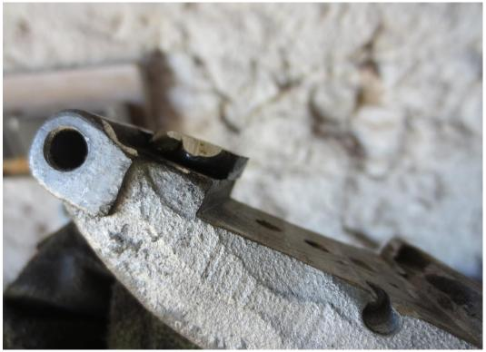
The welded shoulder is at the downstream end of the calliper, thus the torque of the disc will push the pad material against it. As this end is also the fulcrum end of the calliper, wear will be far lower than at the free end, as the pad will wear into a triangular profile with the fulcrum end experiencing the least wear. Therefore there is no danger of this extra shoulder contacting the disc.
