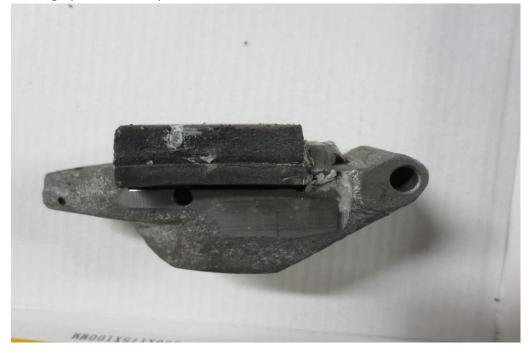
4. Removing as much lost motion from the system as possible and aligning the pad with the disc precisely: The mechanism does not push the pad evenly and squarely against the disc, but in a swinging motion pivoting at one end of the calliper and moving inwards towards the disc at the other. Therefore it is essential to trial fit the calliper arm, with the pad attached, against the disc to ensure a close and parallel pad to disc fit.
