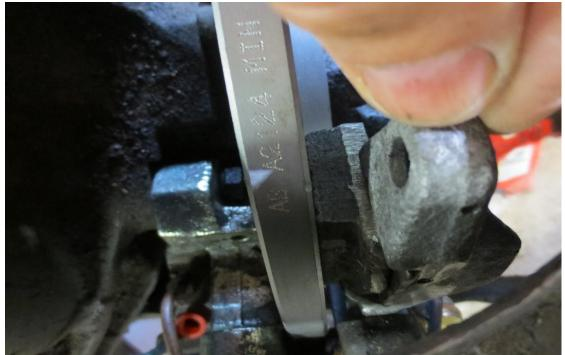
The aim of the trial fit is to then adjust the pad position by using shims (or by sanding down the pad if it is too thick) so that the pad is, at rest, about 5 thou from the disc
