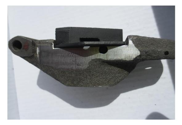
Additionally the pad material was supported by welding an extra shoulder to the calliper which would support the pad material directly, so that the pad-to-backing plate join was not the sole load-bearing surface. Below is a photograph of this modification:
