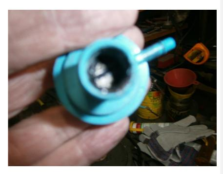
This shows what is under that Mastik plug. Clockwise increases the spring tension.
