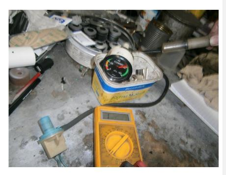
Here, the syringe has applied vac to the switch, and the contacts are Open. Car is cruising down the road. ECU is in Closed Loop mode.
