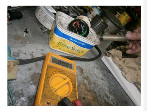
This is the vac reading as the contacts Close, putting the ECU in the Open Loop mode.
