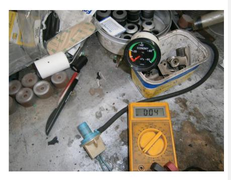
The basic set up I used to establish how this thing worked, and what I needed, to understand the system. Here the vac is Zero, the contacts are Closed. ECU is in Closed Loop mode.
