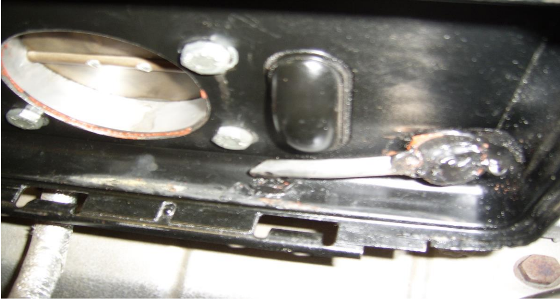
Inside the LH air filter showing the distributor cap vent pipe. A little “rough” looking, but was tidied up later, but forgot to re-snap it.
