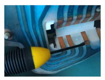
A problem I came across was a broken trace on the top RH (looking from the front) Globe. I repaired this using a bit of solder wick. This is a repair I did 5 years ago and it's still going strong. You could also solder a couple of bits of wire, as long as it touches the globe carrier it should work. Any damaged traces can be repaired with wire as long as it is insulated.
