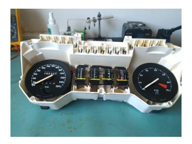
Most problems with intermittent or poor functioning gauges will be caused by the 2 main connectors. It is not uncommon for the traces to detach from the backing causing poor connection. Another common problem is corrosion probably caused by a leaking windscreen at some time in the cars life.
