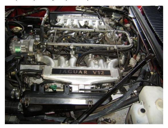
The RED top of the transmission dipstick is visible at the top RH section of the picture, right in front of the brake fluid reservoir.
