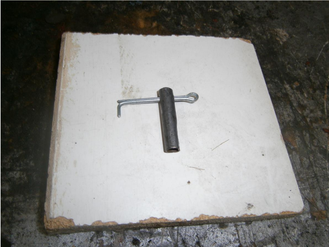
The “tool” made to adjust the ECU potentiometer.
