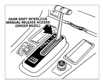
Remove the gearshift lever selector bezel. Gently press down on the interlock release with a screwdriver through the access hole. Move the shift lever out of PARK.
