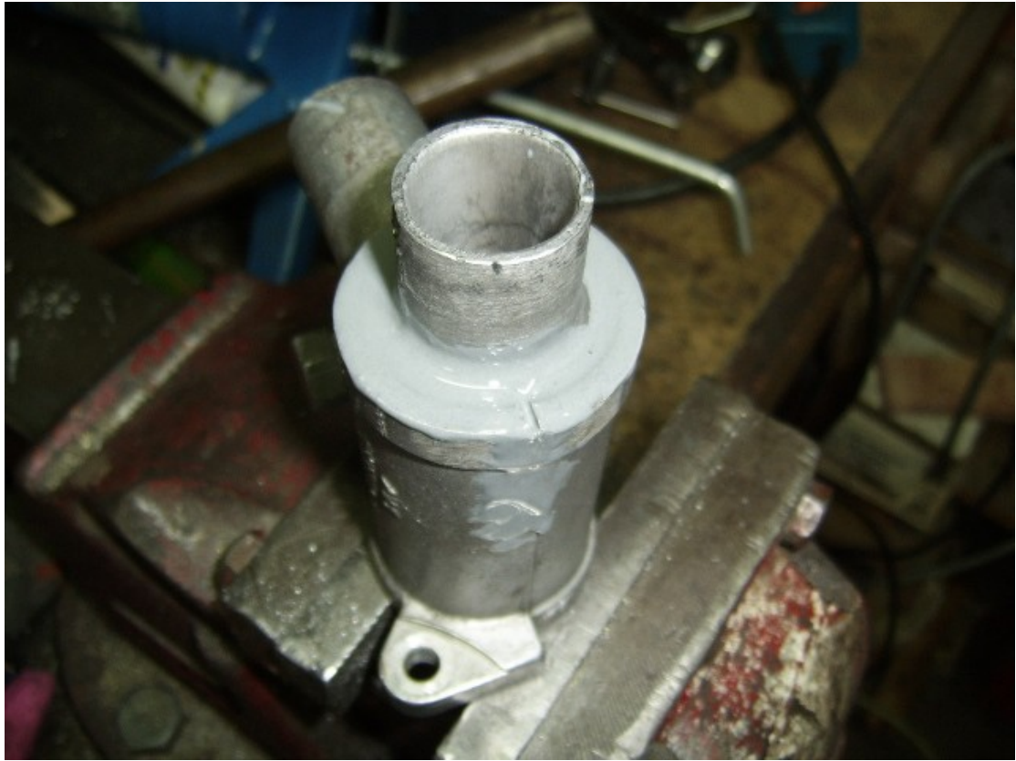
Completed unit with JB weld in place.
