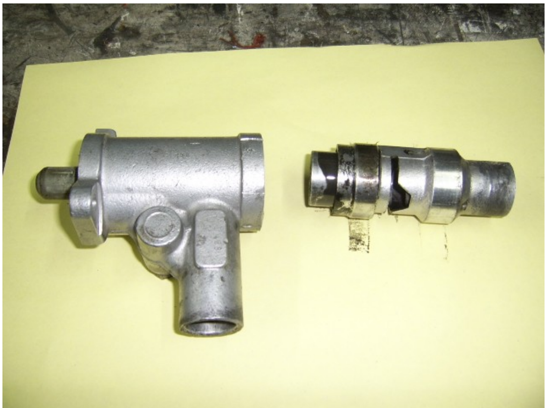
Body on the left and Tophat assembly on the right
