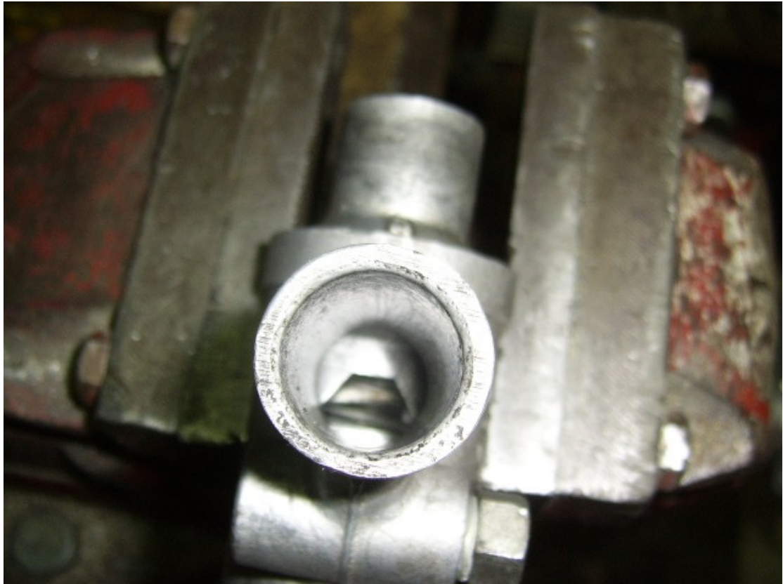
AAV as it is when cold or jammed
