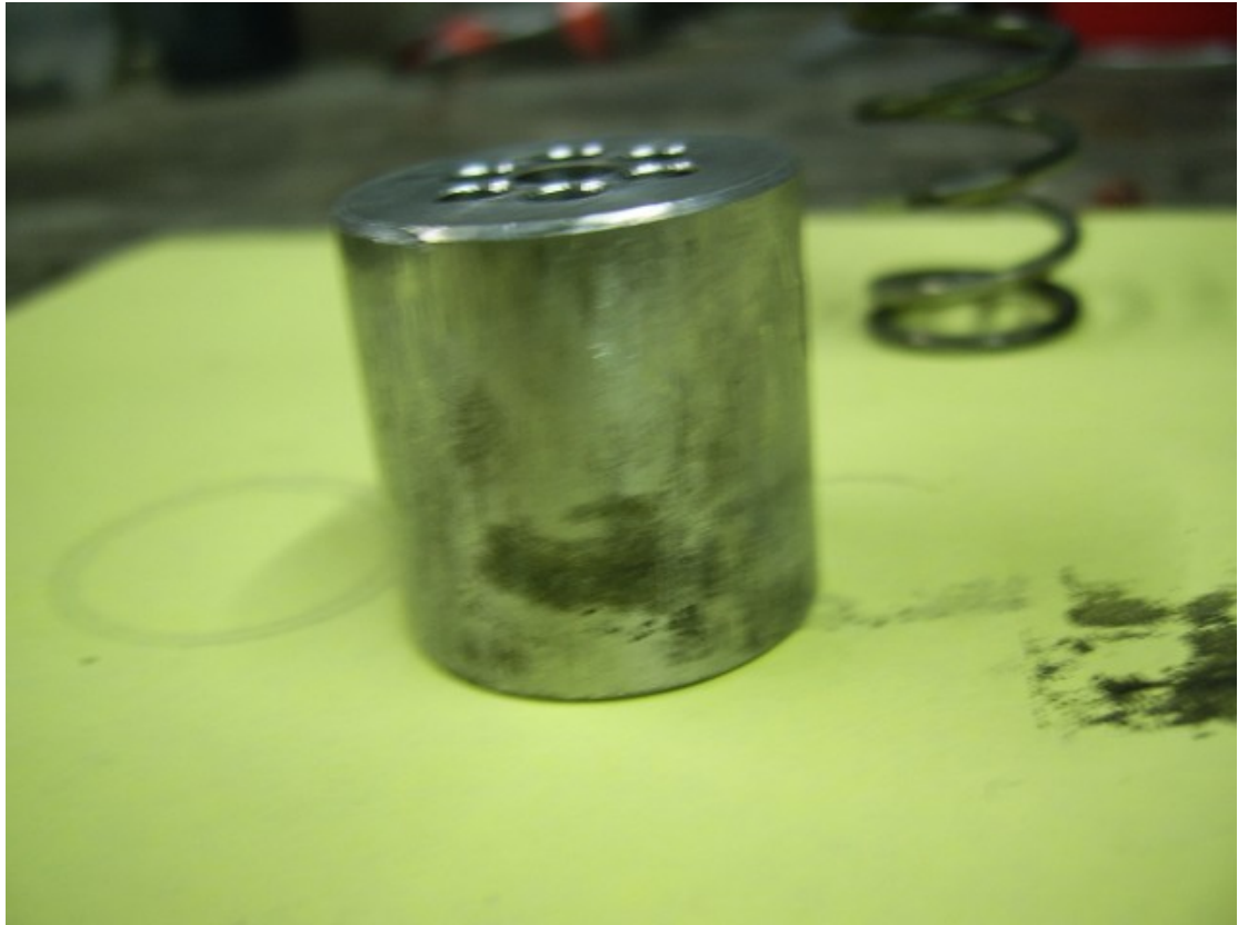
Alloy piston showing scores and carbon build up
