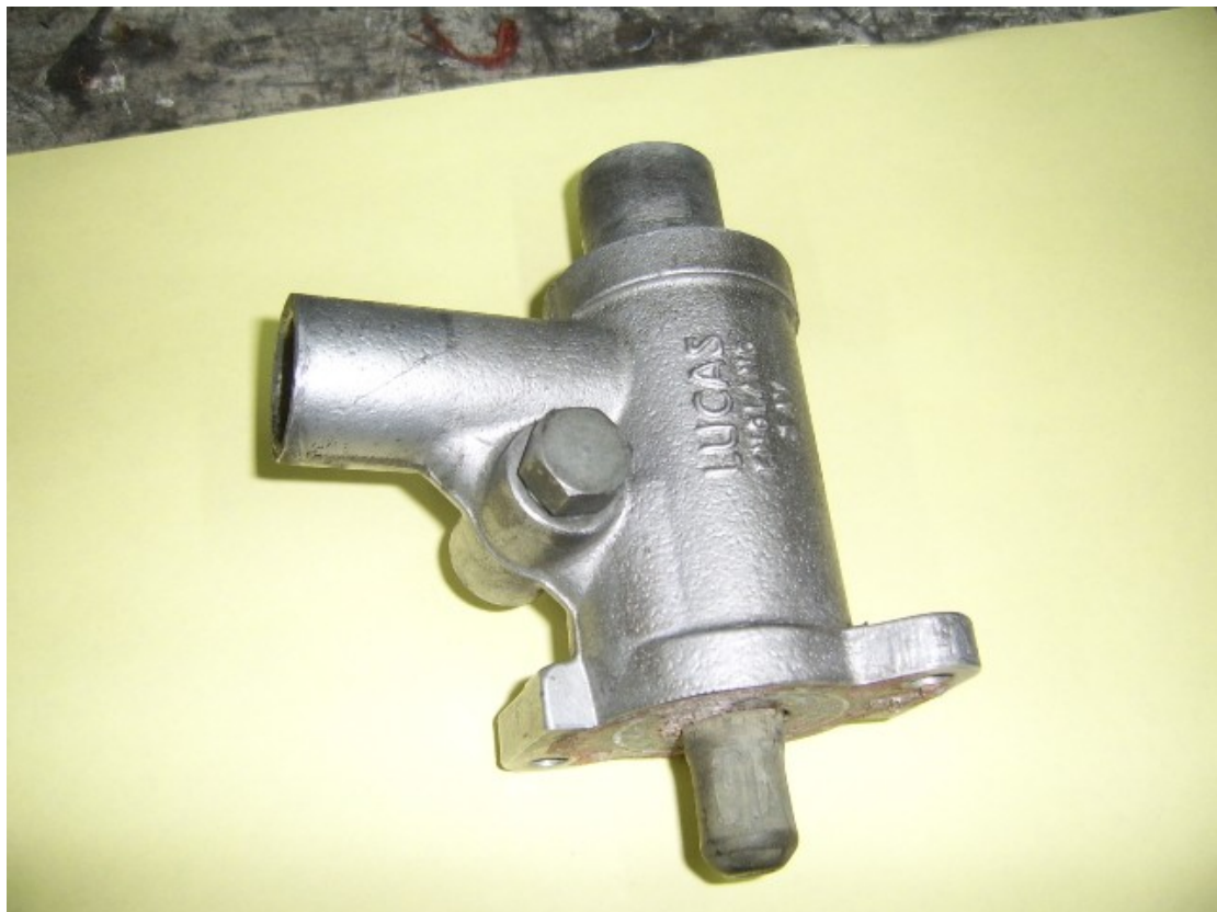
AAV as removed from the engine
