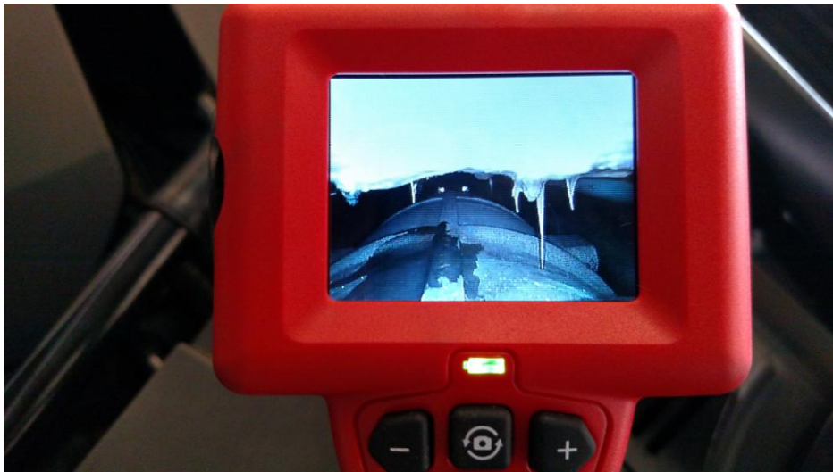
View from camera where water is dropping on transmission.
