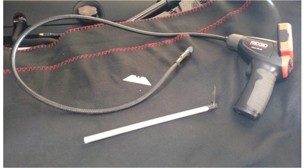
Tools I used; didn't use razor blade just for ref, made knife from a razor blade. Picked up inspection camera from home depot for $79.00 to locate duck bill.
