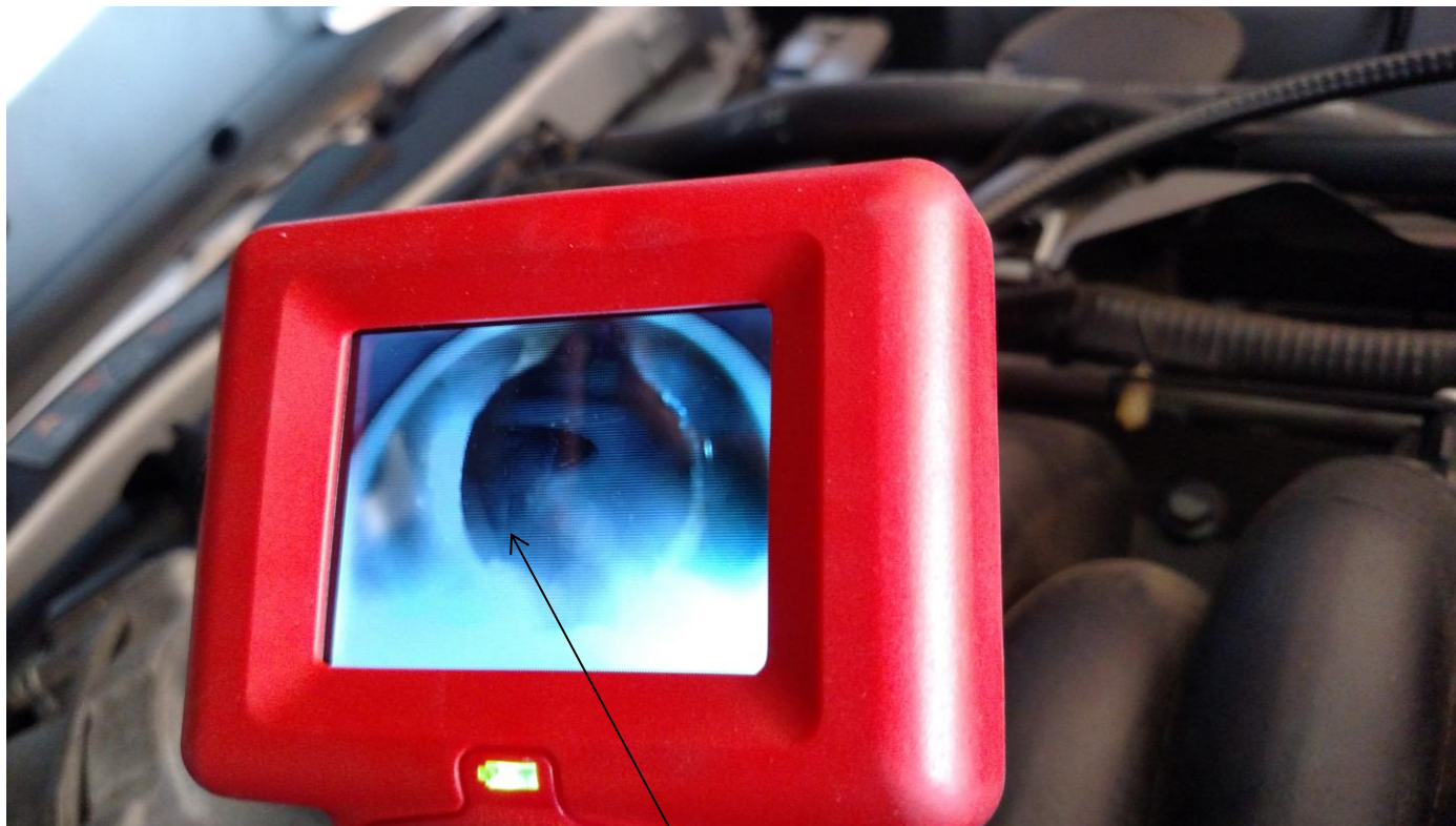
View from camera with mirror attached to look up into hole. After using blade to pry open you can see duck bill is open. Goal was to cut off one half of duck bill but need longer blade to reach. Was able to cut the lower half.
