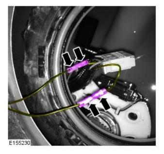
**18.** Using a suitable tool, check the resistance values across fuel tank flange pins listed in the table above.
