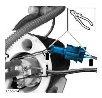
8. Using a suitable tool, remove 5mm of insulation from the end of the 2 wires.
